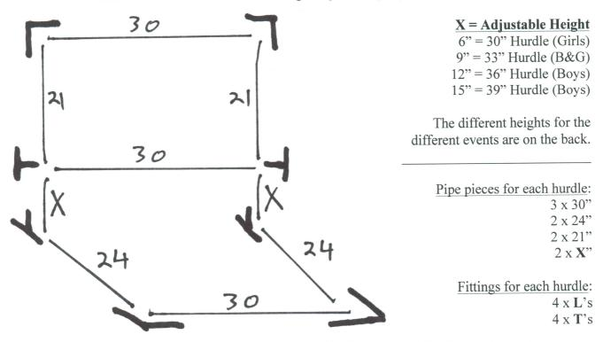
\*For 6 Hurdles, use 24 of each fitting and 10 pieces of 10' ½" PVC pipe, following the cut plan below to give 33" hurdles. The short **X** piece can be changed to vary the height of the hurdle. Color-coding this piece with paint or tape can be helpful if you are making multiple sets for different sizes.
